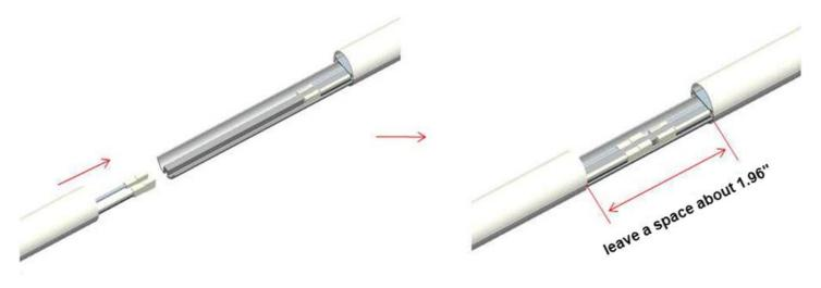
Step 4: Join the ends of the terminal lamp (A) and lamp (B). Press them together tightly.
