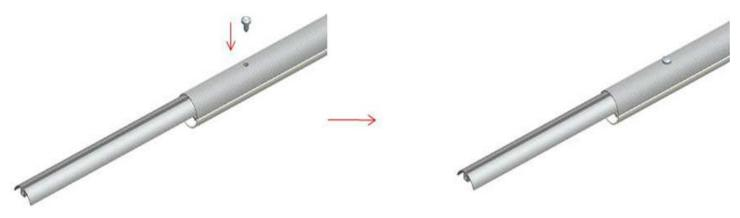
**Step 3:** Take out 4' LED lamp (B) and insert the connected quick connect aluminum into lamp (B). DO NOT insert it completely. Leave a proper spacing (about 1.96") between lamp (A) and lamp (B) for connecting the terminal.
