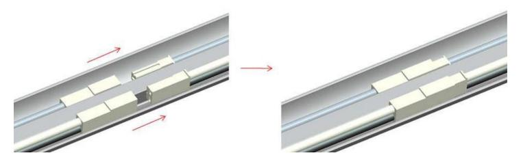
**Step 5:** Press the connected terminal vertically into the slot of the aluminum body so that the upper surface of the terminal is lower than the plane of the connected aluminum body.
